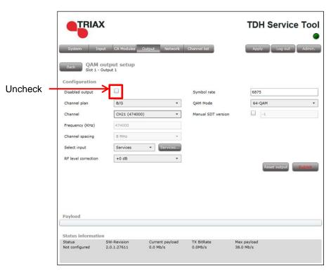
3. Remove the check from the **Disabled output** checkbox.
