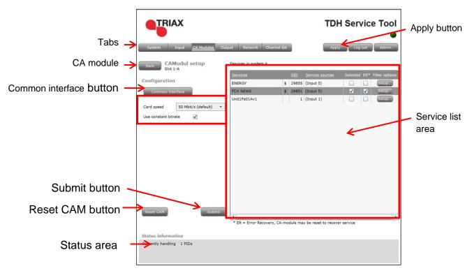
The **CA Module setup** window is displayed, initially containing default values.
