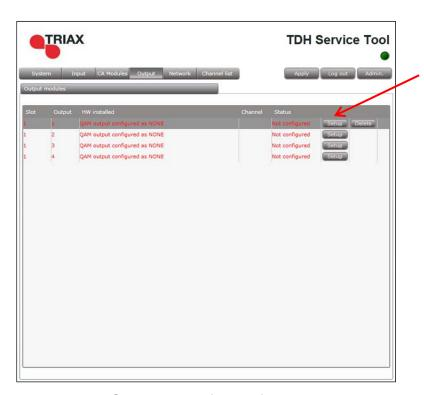
2. Press the **Setup** button for the first output row.
