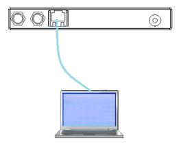
Connect a Cat5e shielded cable or better between the computer's network port and the configuration port on the headend.
