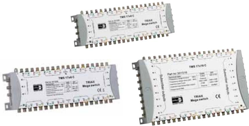
Triax TMS 17x series is an easy-to-install multiswitch system for use where 4 satellite positions are required. A terrestrial input is available to allow terrestrial as well as satellite signals to be available on all subscriber outputs. TMS 17x has an active satellite signal path and a passive terrestrial signal path allowing a terrestrial return path if needed. Satellite position switching is done via DiSEqC signals from the subscriber set-top box.
