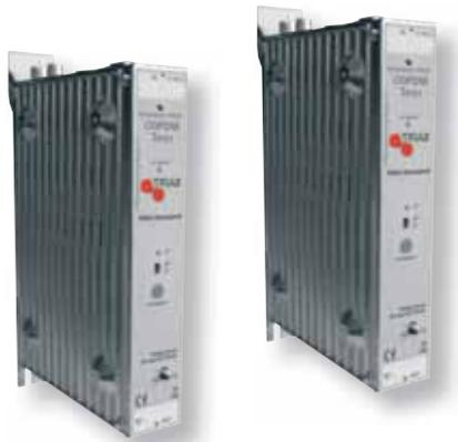
COFDM/RF cross-modulation lines transfer an FTA ("Free-To-Air") programme resulting from a COFDM land multiplex into an HF analogue channel. Sound can be processed in mono or Nicam stereo digital mode. They allow FTA programmes to be broadcasted in a traditional cable television network.
