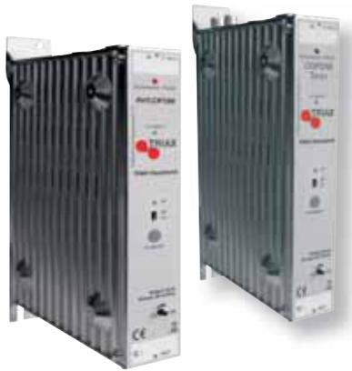
These modules permit distribution of 2 audio video sources (DVD, camera etc..) in the COFDM or QAM formats in an HF network. The signals can then be received by TVs with integrated DVB-T or DVB-C tuners, as well as DVB-T or DVB-C receivers (SD or HD).
