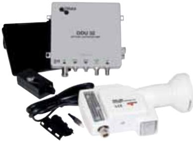
The Triax TDOU216 is a one satellite position optical Ku-Band LNB system that provides a 1310 nm and 1550nm wideband optical output where all eight satellite polarities and a TER signal (DAB/DTT/FM) are stacked into one frequency range (950-5450 MHz) for distribution through one single fibre optical cable. Provides a Link Budget equivalent to  $2 \times 16 = 32$  ways of splitting.
