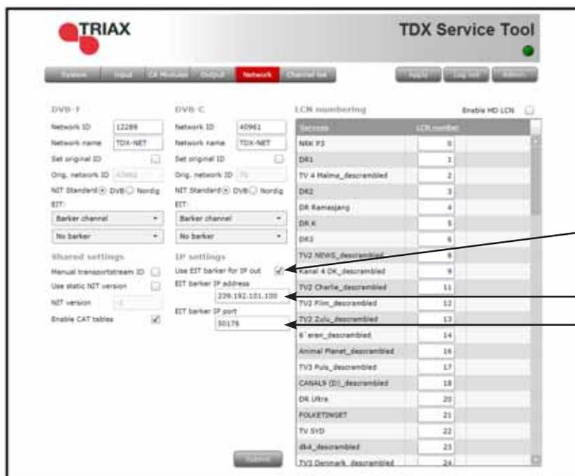
Click the check box to enable the barker channel
