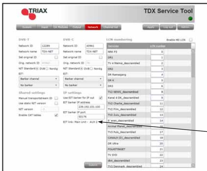
Information about which unit and socket the EIT barker channel uses
