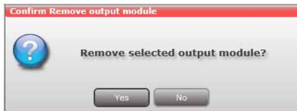
Until you have removed the output module physically from the headend unit, the module list will display four lines with the writing in red.
